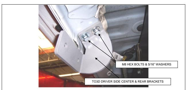
**STEP 5.** Loosely attach the TO3D center and rear brackets, to the body panel using the M8 hex bolts, and 5/16" washers.
