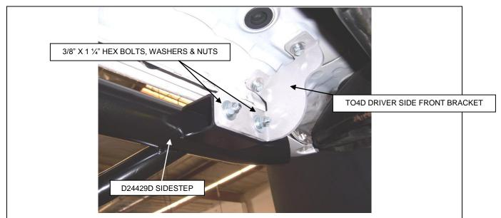
**STEP 6.** Attach D24429D driver side sidesteps to the brackets using the 3/8" x 1 1/4" hex bolts, washers and nuts.
