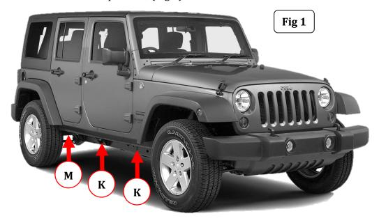
**Step-1** Begin the installation on the passenger side. Starting at the front of the vehicle, locate the holes in the body pinch mold and in the underside of the body, (Fig 2).
