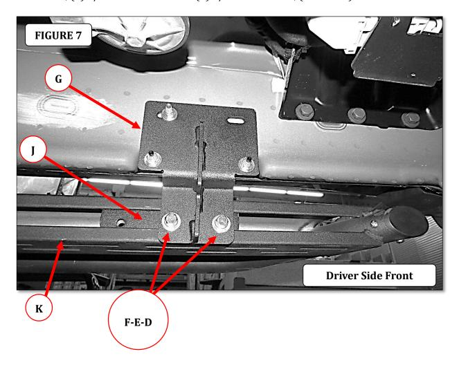
**Step-7** Tighten the nuts securing the brackets to the rocker panel and the bolts securing the Dominator D1 running board to the brackets.
