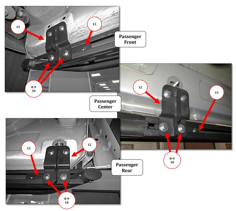
**Step-10** Tighten all bolts securing the Dominator D1 side step to the three side step brackets. Repeat the above steps to install the side step brackets and Dominator D1 side step on the driver side of the vehicle.
