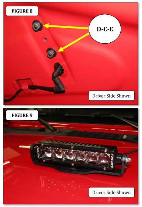
**Step-14** Repeat the above steps to install the LED light and bracket assembly on the passenger side of the vehicle. Re-install the insulator panel to the underside of the hood using the supplied plastic tree clips.
