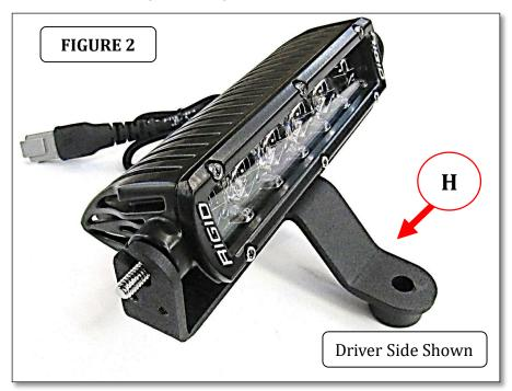
**Step-3** Install (1) retainer plate and (2)  $10-32 \times 1/4$ " button head hex drive screws to each side of the driver side cowl light mount bracket to secure the LED light, then install the flat washers and nylon lock nuts supplied with the LED light, (FIGURE 3). Tighten the screws securing the retainer plates, and snug but do not tighten the nylon lock nuts.
