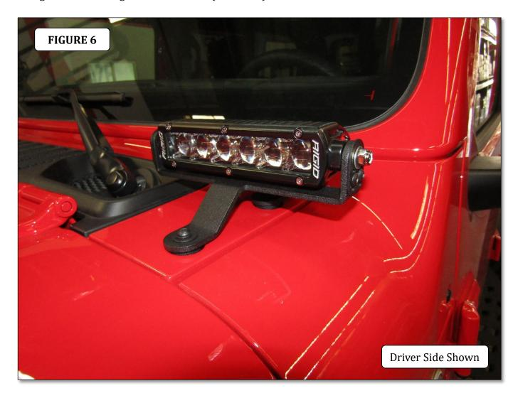
**Step-7** Repeat the above steps to install the LED light and cowl light mount bracket assembly on the passenger side of the vehicle.
