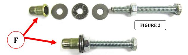
**Step-5** Place the rivet-nut with the attached tool components into the enlarged hole in the body structure. Use a 7/16" wrench to hold the nut, and tighten the bolt using a 7/16" wrench or socket and ratchet. Continue tightening the bolt until the rivet-nut is fully compressed and no longer spins then remove the tool components, (FIGURE 3).
