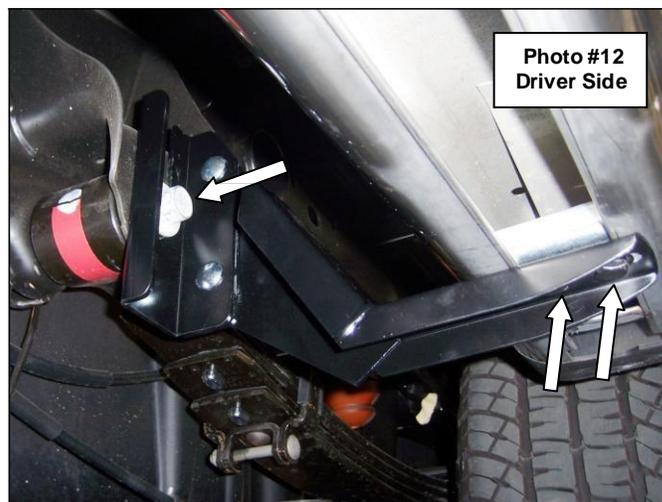
**Step-5** Re-align the side bar with the vehicle and tighten all side bar, bracket and vehicle nuts and bolts.
