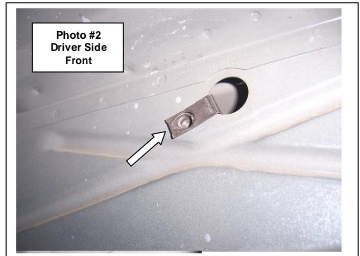
**Step-2** Attach one of the cab brackets to the rocker panel using the u-nut, (1) 3/8" x 1 1/4" hex bolt, (1) 3/8" lock washer and (1) 3/8" flat washer and to the pinch mold using (1) 3/8" x 1 1/4" hex bolt, (1) 3/8" flat washers, (1) 3/8" lock washer and (1) 3/8" hex nut. Leave the nuts and bolts loose for final adjustment. **Photo #3**
