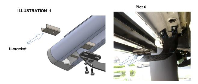
**8.** Align side bar RB10 and then tighten all bolts.
