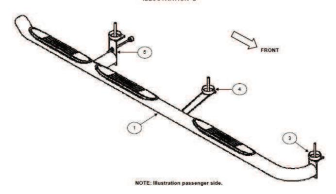
**Step-1** Begin the installation by removing the passenger side front, middle and rear body mount bolts. Keep all existing washers and bushing in place, and attach the front, middle and rear brackets to the vehicle using the factory body mount bolt Leave the bolts loose for final adjustment, (Illustration 3).
