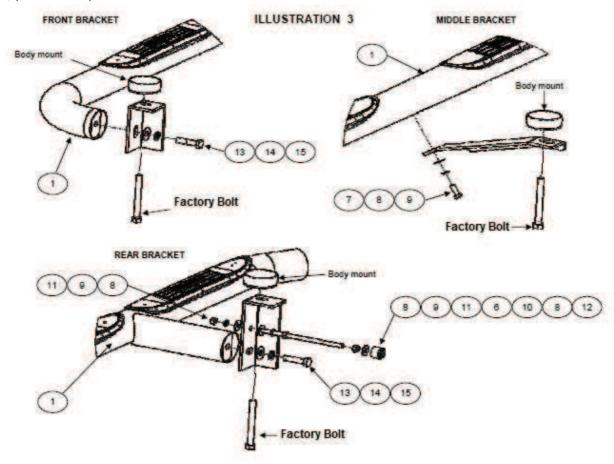
**Step-5** Align the side step with the vehicle and tighten all side step and bracket nuts and bolts.
