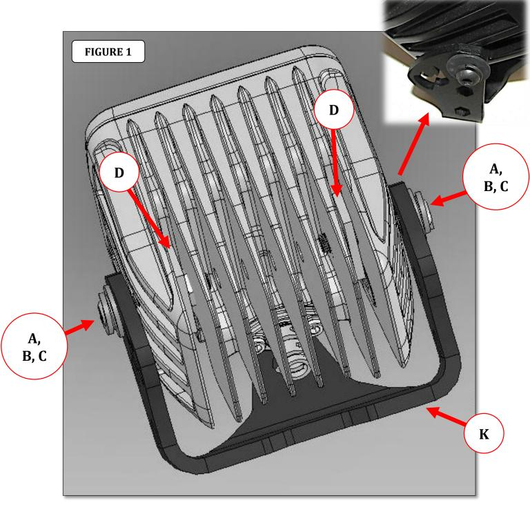
**Step-2** Identify the driver and passenger hard top light mount brackets.
