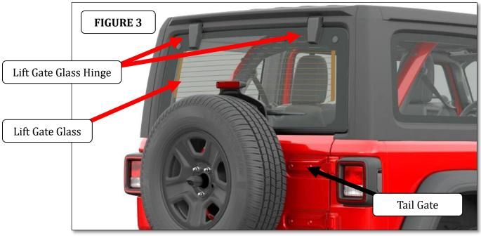
**Step-6** Beginning on the drive side use an M10 socket and remove the (2) hex head screws securing the lift gate glass hinge to the hard top, (FIGURE 4).
