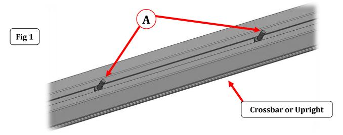
**Step-3** Align the  $\frac{1}{4}$ " x  $\frac{3}{4}$ " hex bolts installed in the crossbars or uprights with the holes in the Overland Series Gear Accessory Plate, and position the Overland Series Gear Accessory Plate on the crossbars or uprights so the  $\frac{1}{4}$ " x  $\frac{3}{4}$ " hex bolts are protruding through the attachment holes in the Overland Series Gear Accessory Plate.
