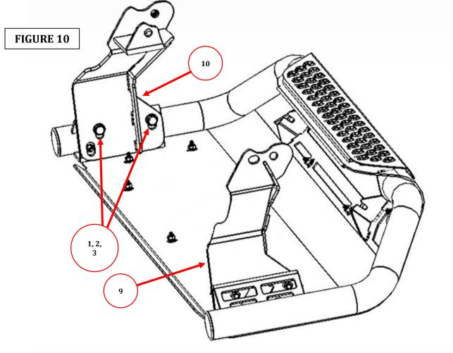
**Step-8** With assistance align and hold the RC3 or RC4 front guard in the desired position on the vehicle, then tighten all OEM and supplied nuts and bolts.
