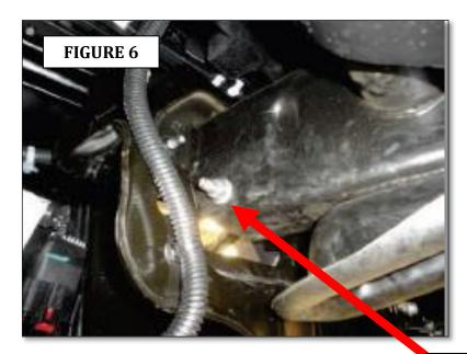
Remove nut and bolts securing the passenger side tow hook to the frame.
