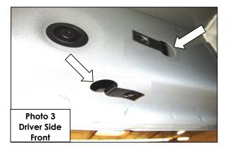
**3.** Attach the driver side front bracket to the rocker panel using (2) 5/16 x 1" hex head bolts, (2) 5/16" flat washers and (2) 5/16" lock washers, **(Photo 4 & 5).** Leave the bolts loose for final adjustment.
