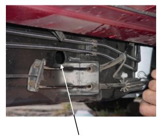
Insert in this hole the 1/2" bolt plate (Driver rear side)
