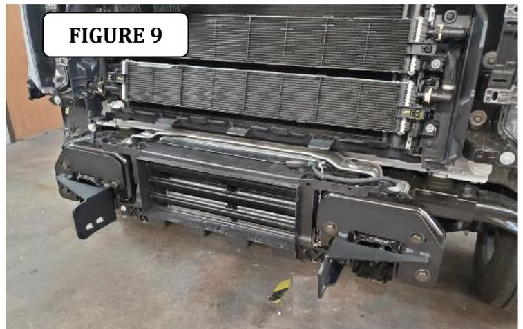
**Step-14** With both brackets installed, leave a center distance of 27 3/4"-28" in between. Brackets should be finger tight to allow for adjustment when installing the center bumper section. Figure 10.
