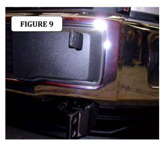
**Step-9** Place the Grille Guard over the brackets. Secure the lower brackets using (2)  $1/2 \times 1 \cdot 1/2$ " hex bolts, (4) 1/2" flat washers, (2) 1/2" lock washers and (2) 1/2" hex nuts. Secure to auxiliary bracket using (1)  $3/8 \times 1 \cdot 1/4$ " hex bolt, (1) 3/8" flat washer, (1) 3/8" lock washer and (1) 3/8" hex nut. Leave loose. Figure 10.
