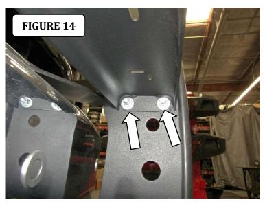
**Step-14** Position the top tube between the grille guard side plates. Attach the to the top tube to the side plates using (2) 3/8" X 1 1/4" hex bolts and (2) 3/8" lock washers (Fig 15). Align the grille guard center section assembly, then and tighten all nuts and bolts for the grille guard center section assembly, winch tray and mounting brackets.
