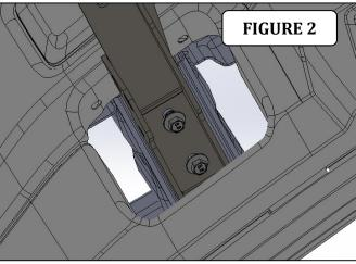
**Step-3** Place the main bracket on the bottom frame . Re-attach using the factory bolts removed in previous step. Figure 2. Leave loose. Follow to step 7.
