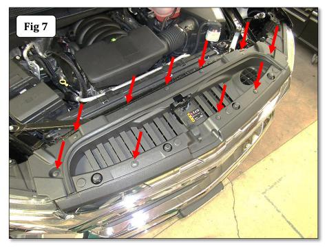
**Step-8** Using a 10mm socket and ratchet, remove the (4) screws (2) per side securing the top of the grille, (Fig 8). Working from side to side, gently pull outward on the grille to unsnap the clips by the head lights, and from the sides and center of the grille. Remove the grille from the vehicle.
