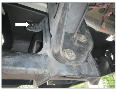
**STEP #8** Align the bumper shell with the vehicle, verify that the tailgate clears when lowered, and tighten all nuts and bolts, (Photo 5).
