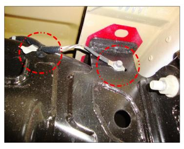
**STEP #3** With assistance support the rear bumper and remove the (3) nuts on each side of the vehicle securing the factory bumper and receiver hitch to the frame. Remove the bumper from the vehicle, (Photo 3).
