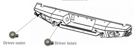
**STEP #4** From the front of the BR20.5 bumper, push the sensor bezels into their precut holes in the sensor bezel brackets. Make sure to install the bezels in the same position and order as the OEM bumper.
