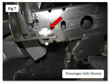
**Step-8** From above on each side of the vehicle, using a 18mm socket remove (1) bolt securing the OEM bumper and bracket assembly to the frame, (Fig 8). Remove the OEM bumper from the vehicle.
