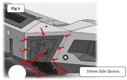
**Step-12** With assistance lift the bumper shell up to the vehicle, align the holes in the bumper shell brackets with the holes in the frame brackets, and weld nuts on the winch tray. Secure the bumper shell bracket to each side of the winch tray using (3)  $\frac{1}{2}$ " x 1 1/2" hex bolts, (3)  $\frac{1}{2}$ " lock washers and (3)  $\frac{1}{2}$ " flat washers, (Fig 7). Leave the bolts loose for final adjustment.
