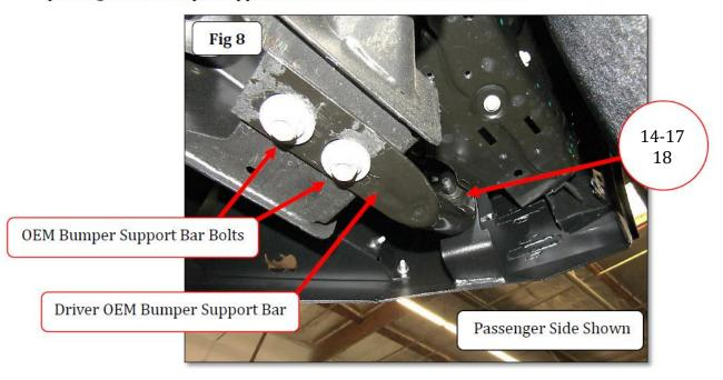
**Step-14** With assistance, adjust and hold the bumper shell visual alignment position, then tighten all factory and supplied nuts and bolts securing the brackets, winch tray and bumper shell. Trim the front fender liners to match the BR6 bumper if desired.
