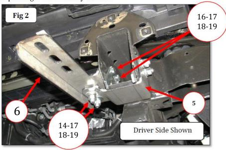
**Step-3** Position the driver side frame bracket up to the end of the frame, align the holes in the frame bracket with the OEM bumper bracket attachment holes in the frame and secure the frame bracket to the frame using (2) of the OEM bumper bracket bolts, (Fig 3). Leave the bolts loose for final adjustment. Repeat to install the passenger side frame bracket.
