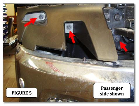
**Step-8** On each side of the vehicle, remove (2) bolts securing the bumper valance center support bracket, (FIGURE 6). Remove the valance center support bracket from the vehicle.
