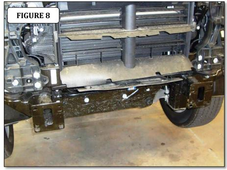
**Step-11** Reinstall the factory grille and radiator dust cover.
