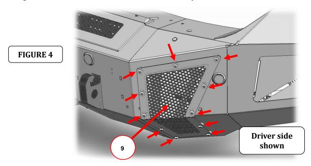
**Step-5** With assistance lift the bumper shell up to the vehicle, align the holes in the bumper shell brackets with the holes in the frame brackets, and weld nuts on the winch tray. Secure the bumper shell bracket to each side of the winch tray using (3)  $\frac{1}{2}$ " x 1 1/2" hex bolts, (3)  $\frac{1}{2}$ " lock washers and (3)  $\frac{1}{2}$ " flat washers, (FIGURE 5). Leave the bolts loose for final adjustment.
