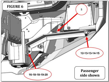
**Step-7** With assistance, adjust and hold the bumper shell visual alignment position, then tighten all supplied nuts and bolts securing the brackets, winch tray and bumper shell.
