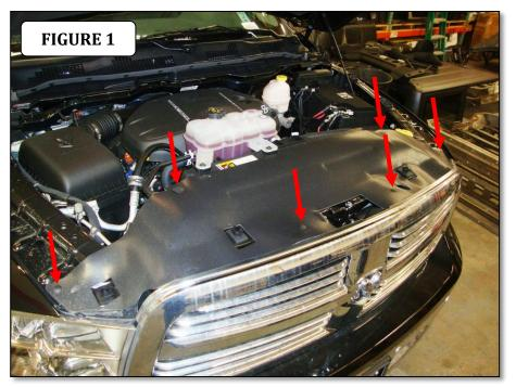
**Step-3** Remove the (4) screws securing the top of the grille to the radiator support, (FIGURE 2). Unsnap the pins located behind the grille on each side midway and bottom, and then remove the grille from the vehicle.
