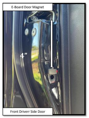
Step 17: FRONT DOOR Apply a vertically oriented strip of masking tape on the front Driver side door using the deepest part of the latch as a reference point. Make a mark 3.5" below the center line of the latch. Prepare the surface by cleaning with a 50/50 mix of isopropyl alcohol and water or equivalent. Once the surface is completely dry, peel the backing from the double-sided tape and stick the magnet to the door. Align the top of the magnet with the 4" mark as shown.
