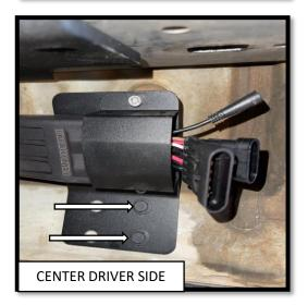
**Step 5**: Install the CONTROL MODULE on Passenger side center mount side motor using (2) M8X25mm Flange Bolts.
