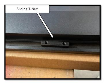
**Step 6**: Install the PASSENGER side running board. With assistance, begin by positioning the board on the front and rear motor assembly bases. Align the sliding T-Nut on the running board with the slots on the front and rear motor base. Once the T-Nuts are aligned, rotate the running board so that the T-Nuts set in the slots on the base of the arms. Repeat 1-7 to install the motor linkage assemblies and running board on the DRIVER side side.
