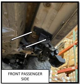
**Step 4**: Install the FRONT PASSENGER side motor using (2) M8X30mm Flange Bolts, to fasten the motor to the vehicle. The hardware should be hand tightened only until snug. This will allow the motor assembly to move and align easier when installing the running board.
