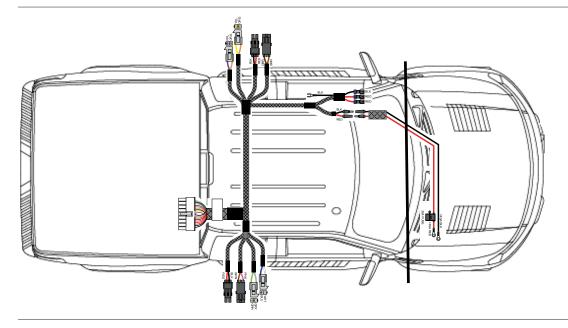
Lift the carpet behind the front seat and locate and remove the vent plug. Route the driverside actuator (red/black) and LED light (brown/ tan) wires through the floor and outside of the vehicle. Reinstall the vent plug.
