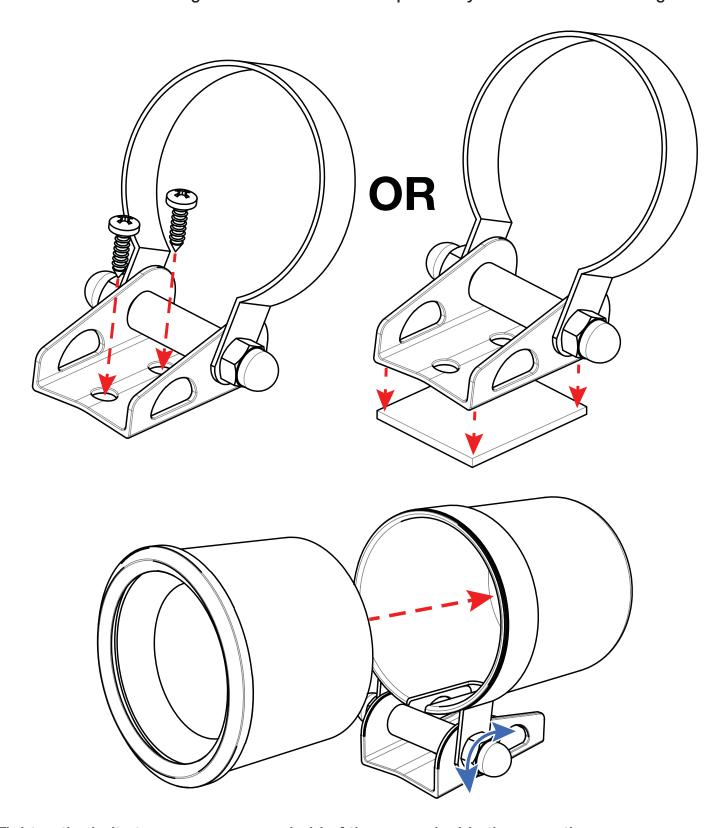
Tighten the bolts to ensure a secure hold of the gauge inside the mounting cup.
