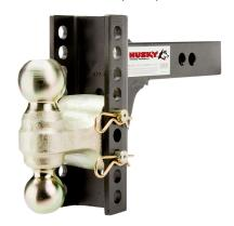
The DFB is rated up to 10,000 lbs. GVWR/1000 lbs. tongue weight when using the 2" ball and 14,000 lbs. GVWR/1,400 lbs. tongue weight when using the 2-5/16" ball.
