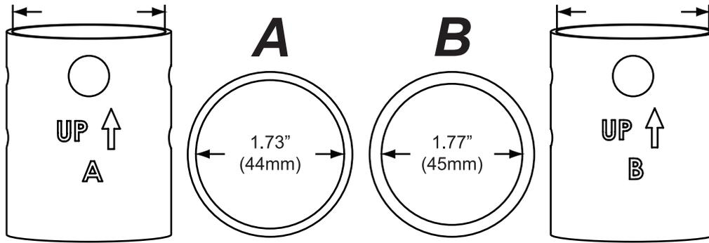
These bushings are designed for use with jacks that have 2" inner tubes. Bushing A is a general purpose bushing to fit 2" jacks. Bushing B is specifically designed to fit 2" Husky electric jacks, which have slightly smaller inner tubes. Install the appropriate bushing over the end of the inner tube of your jack, aligning the side holes of the bushing with the holes at the bottom of the inner tube.
