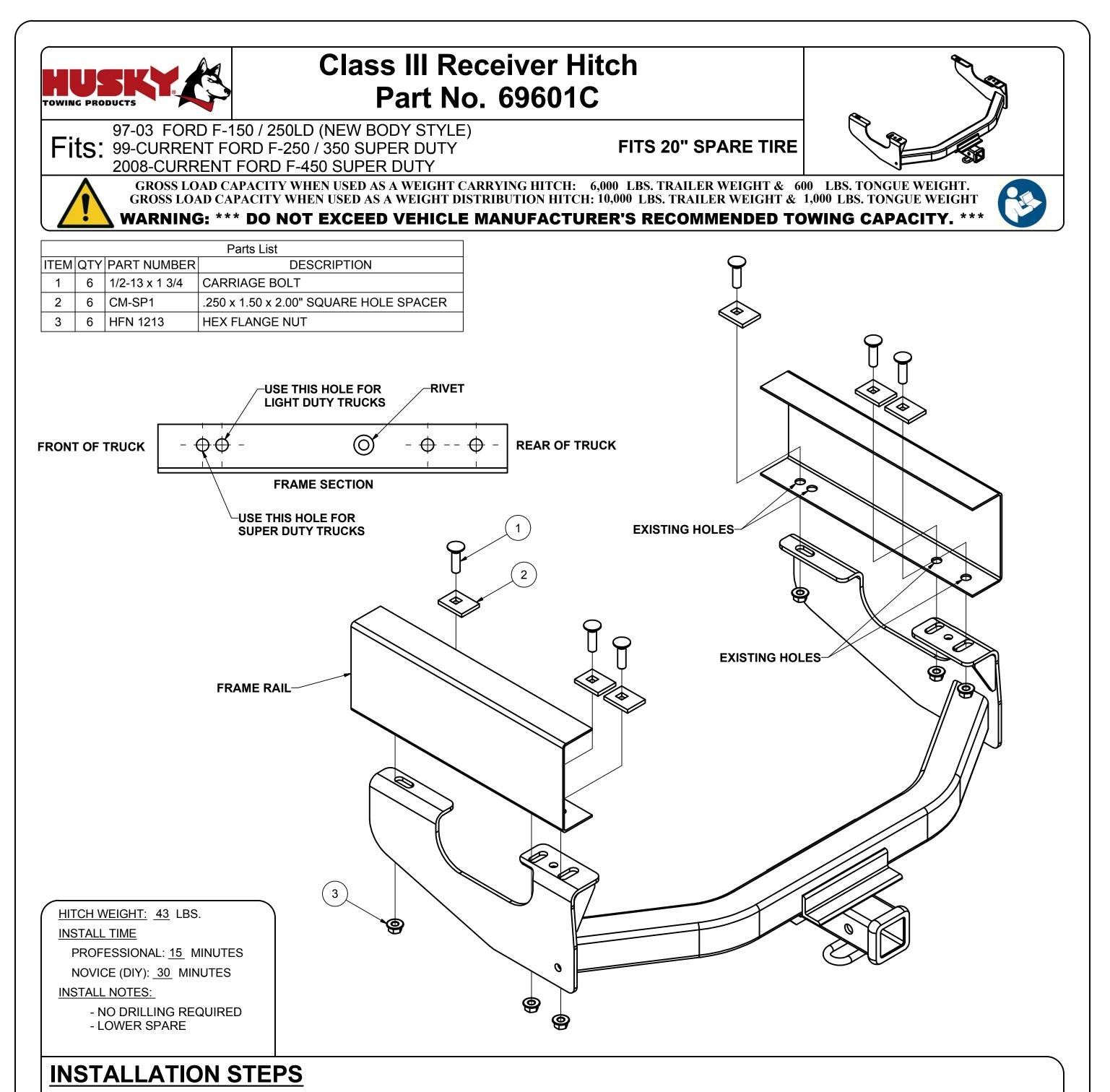
1) Lower the spare for ease of installation. (Spare will be replace after hitch is installed.)
