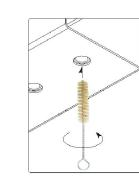
WELDNUT CLEANING To remove debris from weldnuts in frame, spray lubricant or
