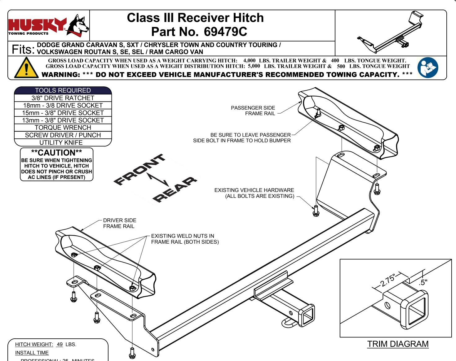
PROFESSIONAL: <u>25</u> MINUTES NOVICE (DIY): <u>50</u> MINUTES <u>INSTALL NOTES:</u> - NO DRILLING REQUIRED - USE EXISTING FASTENERS - LOWER EXHAUST
