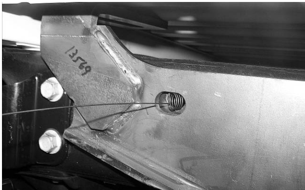
Insert pull wire through slot in bracket.
