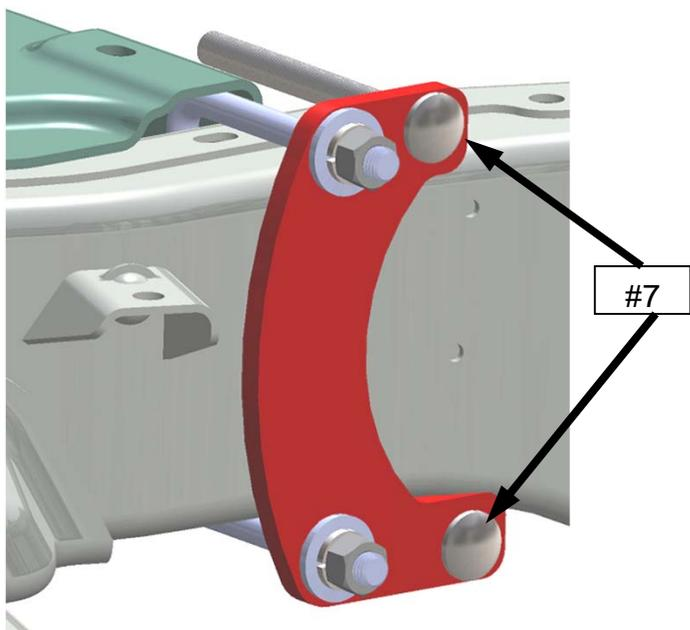
8. Slide spacer tubes (#12) over carriage bolts (#7). See Figure 8.
