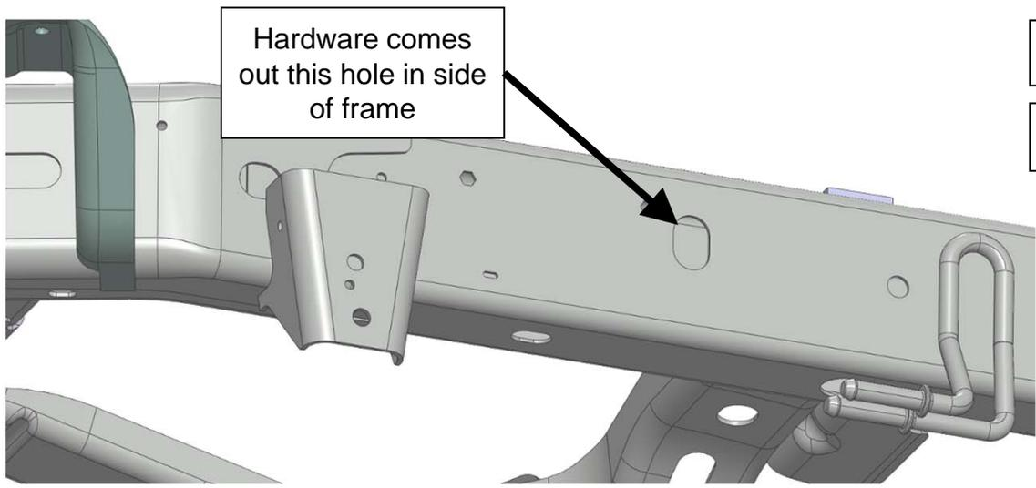
16. Align the rear base rail with the holes drilled in steps 16. Use the 5/8" Hex head bolts (#14), 5/8" flat washer (#15) & 5/8" Lock washer (#17) to attach the rear base rail to the rear brackets installed in step 16. Re-measure your base rails as in Step 2. Once you are sure everything is square; hand tighten the 5/8" hardware first. Then tighten and torque the 1/2" hardware on the rear brackets to 75 ft. lbs.
