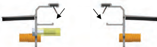
Figure 7—Ensure rails are level
