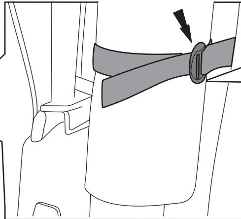
**Note:** Straps should be snug and can be tighten later for the tonneau cover to properly mount.
