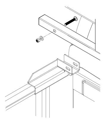
Fasten Backrack to the Rail mount bracket, or Toolbox bracket. Finger tighten at this stage. Center rack on truck and fully tighten both carriage bolts, and 3/8" rail mount bolts. Tighten 3/8" nut to secure.
