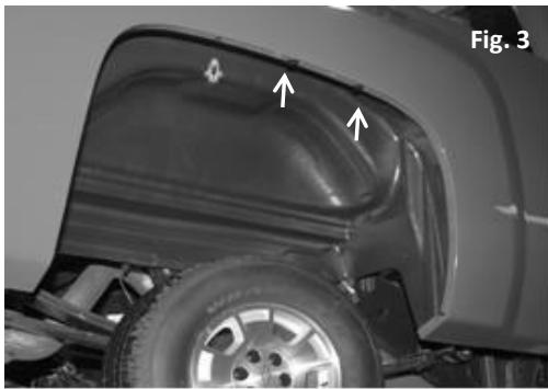
5. Using a drill with socket/driver 5/16" (7mm), Install one self-taping screw in each pre-drilled hole of the plastic liner and into the wheel house sheet metal . (See fig. 4 and 5)
