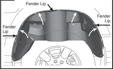
Locate the (2) pre-drilled holes 1 & 2 in the plastic liner. Install fastener saved in step 4 in front hole 1. Install one of the push lock pins (C) provided in rear hole 2. Note: Make sure all holes
