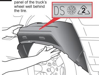
Tuck the lower cab and tail part of the wheel well liner behind the metal lip of truck's fender.
