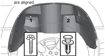
Only replace factory fasteners 1-4 & 8-11 that you removed in step 5 with a 5/16" socket and driver.
