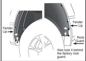
8 Tuck the upper part of the wheel well liner behind the rest of the metal lip of the truck's fender.
