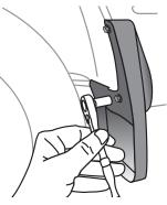
Start on the driver's side and locate factory fasteners 1 & 2 that hold the front and rear molding brackets to the sheet metal.
