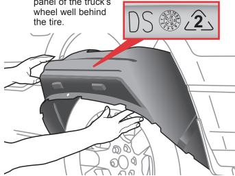
Tuck the lower cab and tail part of the wheel well liner behind the metal lip of truck's fender.
