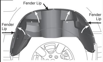
Locate the (2) pre-drilled holes 1 & 2 in the 9 plastic liner. Install fastener saved in step 4 in front hole 1. Install one of the push lock pins (C) provided in rear hole 2. Note: Make sure all holes
