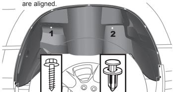
Tighten the factory fasteners 1-8 that you loosened in step 5 with a 5/16" socket and driver.
