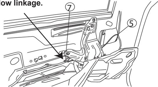
**29** Reassemble door and replace plugs. Plugs must be replaced for Power Step to operate.
