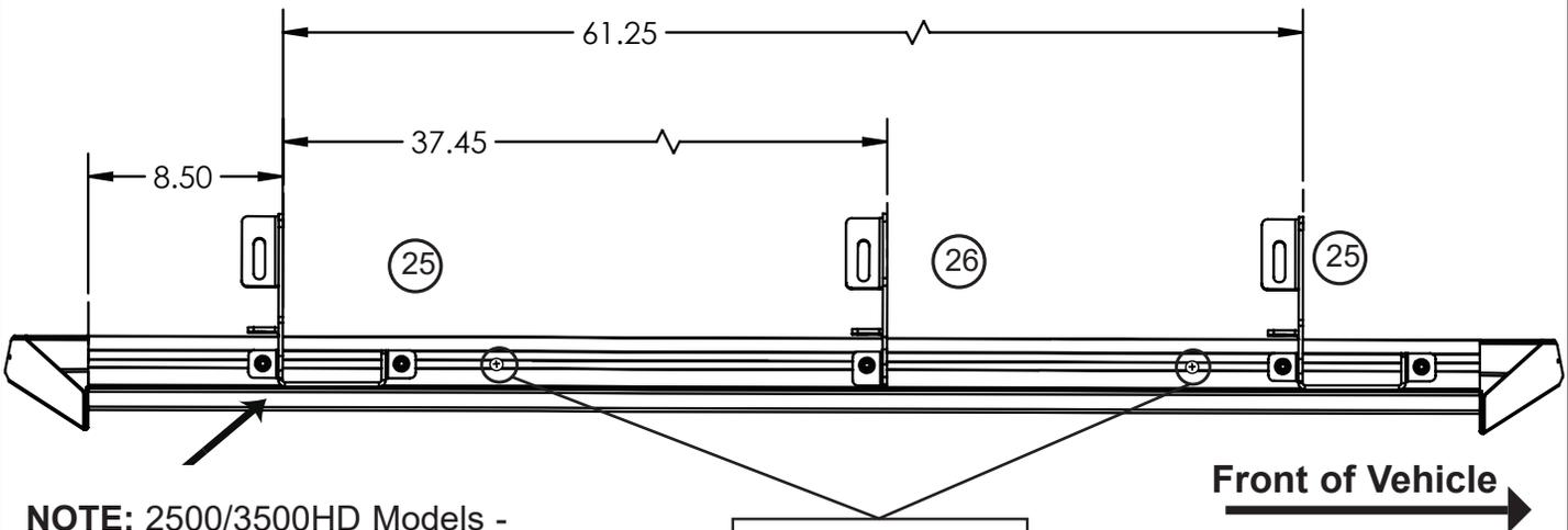
**NOTE:** 2500/3500HD Models - Rear mount on passenger side of vehicle will need to be moved forward from last mounting hole to second to last hole. Approx 15-1/4".
