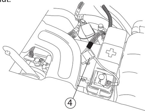
12 Attach ground lead to negative battery pole.
