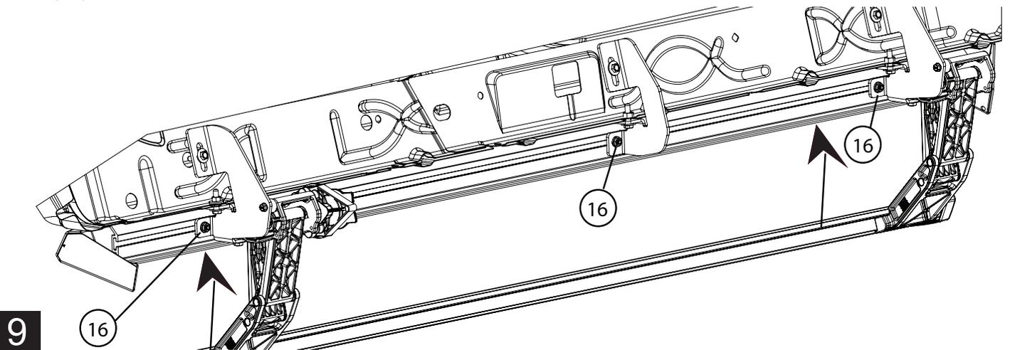
**A:** Using a 13mm socket tighten 3 bolts along pinch weld first. Torque to 16ft-lbs.
