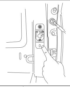
Place Mounting Bracket aligned with top hole. Allow bracket to hang vertically. Mark (Center Punch) location of lower hole using the bracket slot as a template. Remove bracket. Drill hole with 1/8" drill bit then drill out hole with 21/64" drill bit. Use file to remove burrs. Apply primer to edge of hole. Allow primer to dry.
