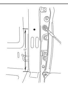
Remove the 2 Phillips screws that are holding the tail lights in place. Carefully pull back to remove tail lights.
