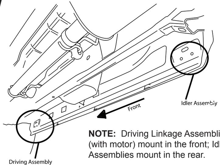
**NOTE:** Driving Linkage Assemblies (with motor) mount in the front; Idler Assemblies mount in the rear.
