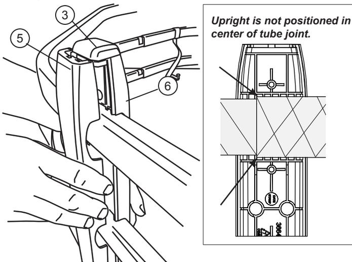
**NOTE:** The inside of the upright is stepped to fit correctly around the small and large diameter tubes.
