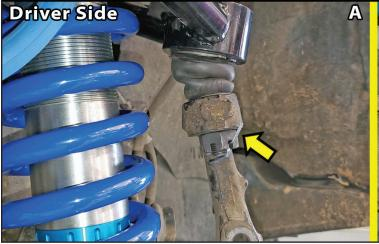
14. REATTACH BRAKE LINE BRACKET TO KNUCKLE... [Illustration 14]
