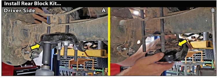
**[Illustration 24-A & 24-B]** The lift block is flat. Position the SUPERLIFT block #028 on top of the axle pad.
