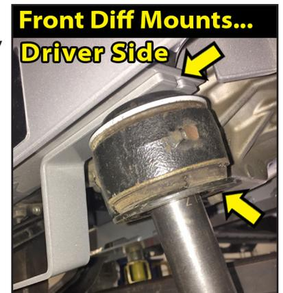
**[Illustration 20-B]** Once Driver side bolt is in place; install the rear differential support bracket (55-37-8200) over the bolt, then install the 18mmn washer and Nyloc nut.
