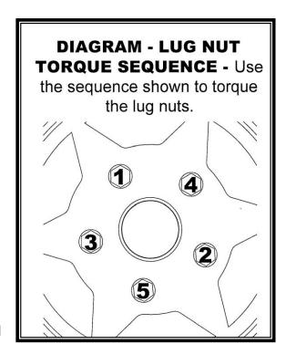
wheel mounting surface (hub, rotor, etc.). Installing wheels without the proper metal-to-metal contact at the wheel mounting surfaces can cause the lug nuts to loosen and the wheel to come off while the vehicle is in motion.
