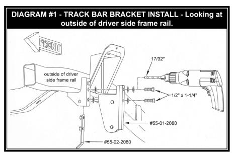
☐ Install the supplied 1/2" x 1-1/4" bolt and 1/2" SAE washer through the "01" bracket and factory bracket. Slide the supplied tab nut (#55-02-2080) between the frame and factory
