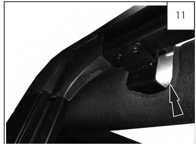
11 Position door surround rear bracket onto the vehicle and fit the bracket over the sport bar.
