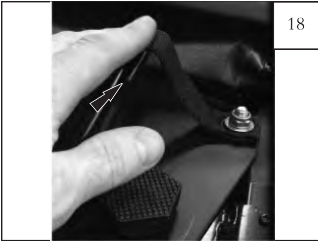
When the top is in the folded back position reach up and hook the retention strap over the bar as shown. Note: The strap is used to safely secure the soft top in the open position at high speeds.
