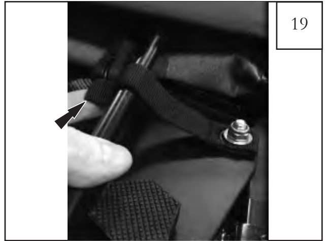
Make sure to unhook the retention strap from the bar before folding the top forward again.
