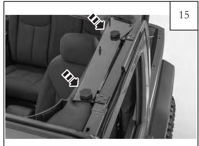
Starting at the front bracket hole insert door surround knob into hole and tighten. Repeat step 14-15 for other side.
