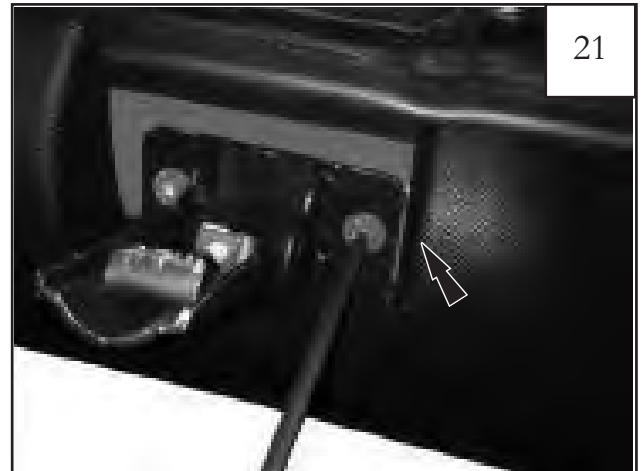
Install provided latch as shown and reattach with the Torx T25 bolt from the previous step.
