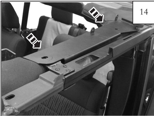
Place driver side mount plate on top completed door surround onto the vehicle and fit the bracket over the roll bar. Line up front hole to the front bracket door surround. Repeat this step for both sides.
