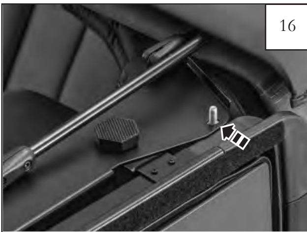
Fit top retention strap to door surround mount plate hole located at rear. Locate the unused hole on the back of door surround plate as shown. Note: There is only one strap and it is installed on the driver side.
