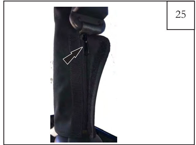
Locate zippers and connect and start zippers as shown on each side.
