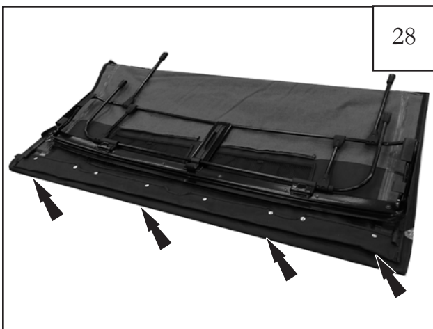
Place the top hardware tubes assembly on top of the main deck fabric then insert into the front pocket. Secure with snaps as shown. Tip: Place front metal into corner pockets and pull all the way until it fits snug.
