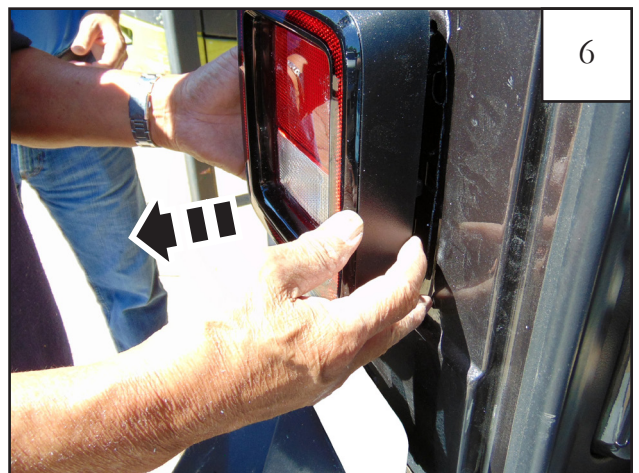
Carefully pull the tail light assembly away from the vehicle.
