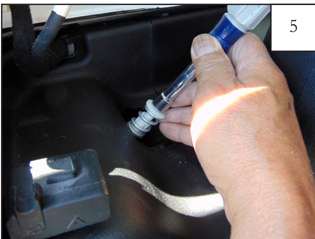
Use a 10mm nutdriver to remove the tail light retaining bolt.
