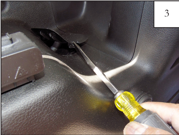
Use a screwdriver to pry open the cover for the tail light retaining bolt.
