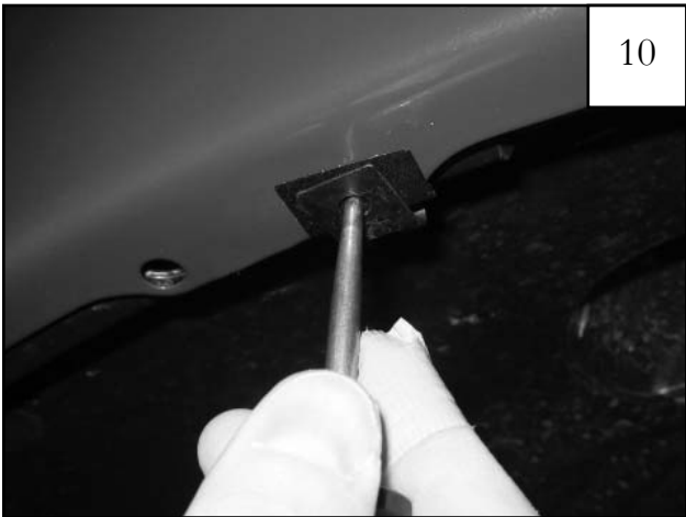
Using an awl or similar pointed tool, poke a hole through Tab (MT1-0014) using the Clip (CL1-0022) hole as a guide.
