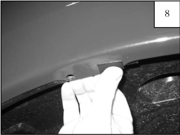
Install Tab (MT1-0014) over existing factory hole. There are two holes at the top center location. Refer to step 7 for proper hole for installation.
