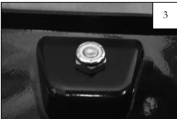
Place a Nut (NU1-0019) over the end of each Bolt and tighten, using a 1/2" wrench for the Nut and the supplied Torx Bit (SW1-0052) for the Bolt. Repeat for remaining pockets.
