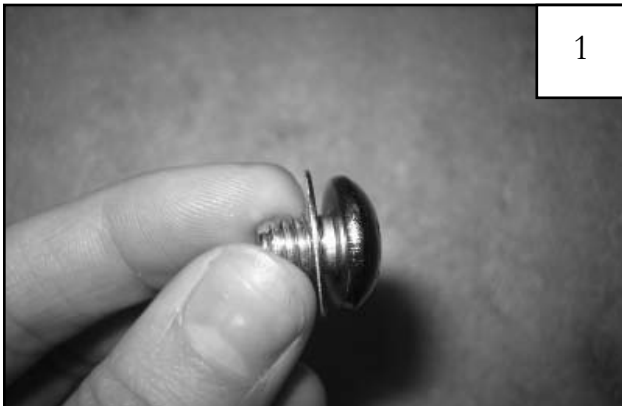
Put a Washer (WA1-0012) on each Bolt (SW1-0067).
