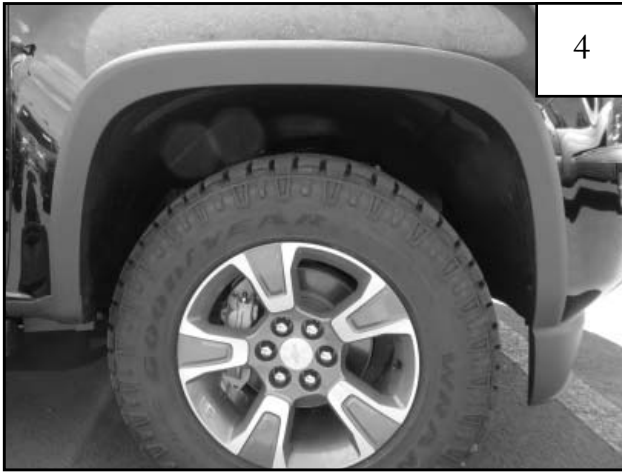
Fitment Note: If factory flares are installed, remove before starting installation. Factory fasteners require a T-15 torx bit.
