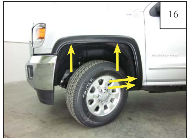
16 While holding Flare on vehicle, install supplied screws (SW1-0056) into the two upper and lower factory holes locations. Do not fully tighten at this time.
