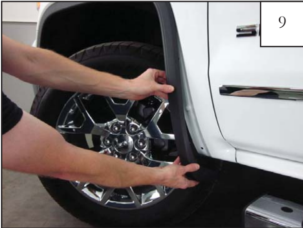
Starting at the lower rear end of the factory wheel arch molding, firmly grip part and pull to remove from vehicle. Note: You will hear popping sounds as the factory fasteners release from vehicle. This is normal.
