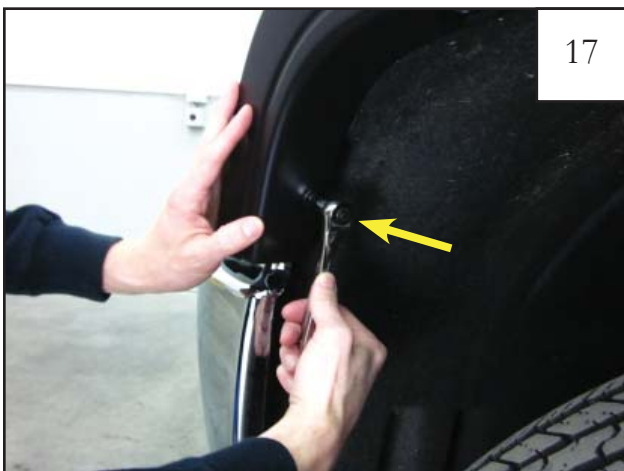
17 While holding Flare on vehicle, install factory screw removed in Step 4 through flare and into factory hole. Do not fully tighten at this time.
