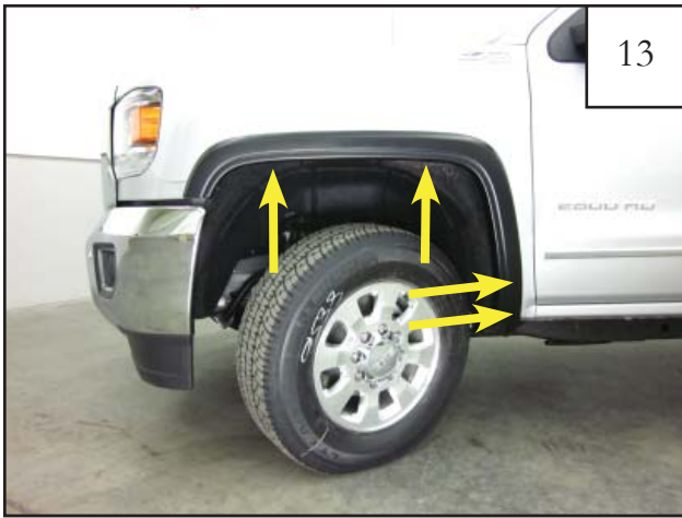
13 While holding Flare on vehicle, install supplied screw (SW1-0056) into the four factory hole locations as shown. Do not fully tighten at this time.
