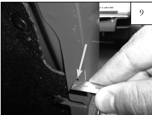
Remove the flare. At the marked location made in Step 7, measure inward 10mm from the edge of the fender and mark with grease pencil or marker. These are the marks to be drilled.
